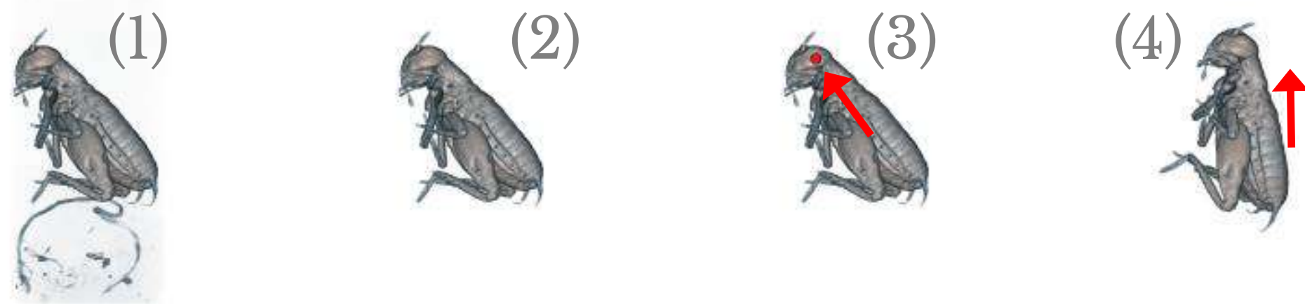
Figure 1 – Overview: 2D rendering of raw (1) and segmented CT (2). Detection of head (3) across multiple views to estimate 3D main axis, enabling specimen reorientation (4).
